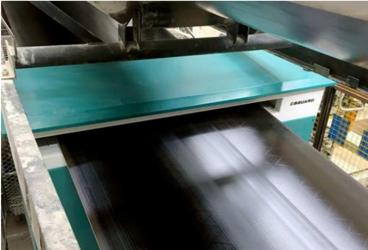
The monitoring technology of the CBGuard system generates a constant video feed of a scan that penetrates the conveyor belt and notifies the operator of problems.
